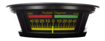
TRI-2 is applied for the indication of the rudder position on the bridge. The indicator consists of a robust moving coil system equipped with three pointers mounted on a common shaft. The TRI-2 is available with CAN or analogue input.
