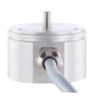
DEIF's rudder/azimuth angle transmitters convert the rudder or azimuth thruster's position angles into either electrical current signals or digital data values with a 16 bit resolution (+/-180de.g. = +/-32767).
